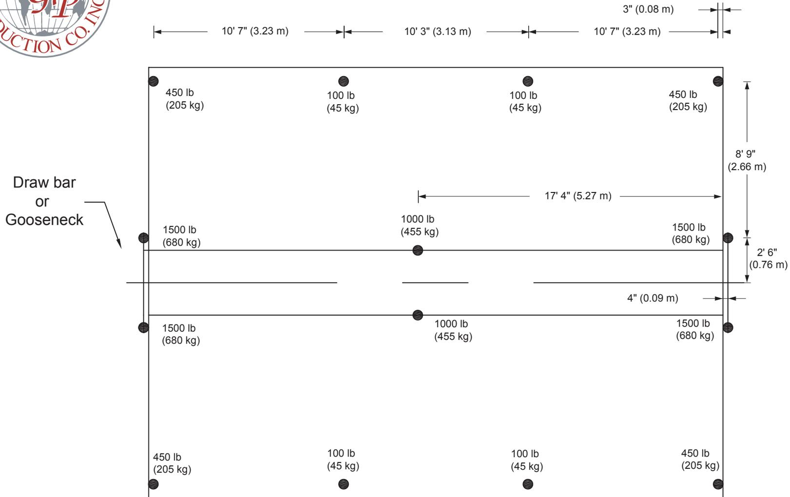
● : Floor stabilizers, extension and levelling jacks.
